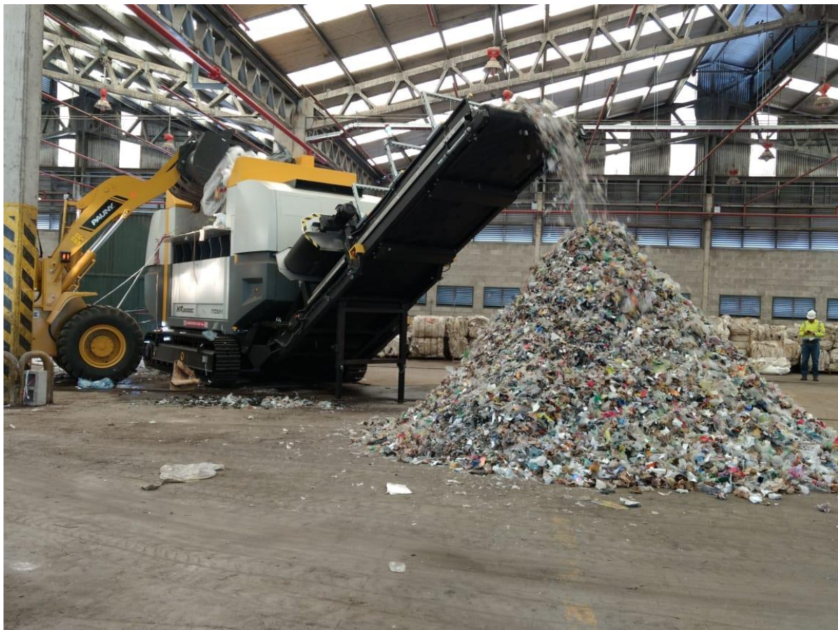
Figure 2. A simple waste shredding operation which produces fines as a residual waste material after sorting.
